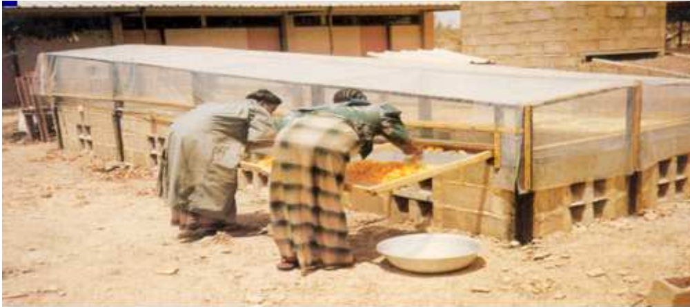
Figure 17. Séchoir solaire tunnel banco.
