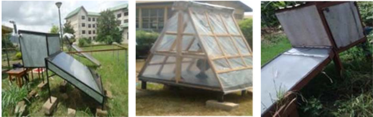
Figure 8: a) Mixed mode solar dryer at Koforidua Polytechnic, b) Direct solar dryer and c) indirect solar dryer
