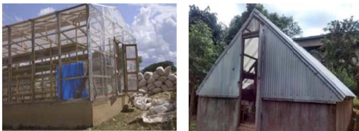
Figure 11: a) Tent type solar dryer at Sekyedumase and b) house solar dryer at Mampong
