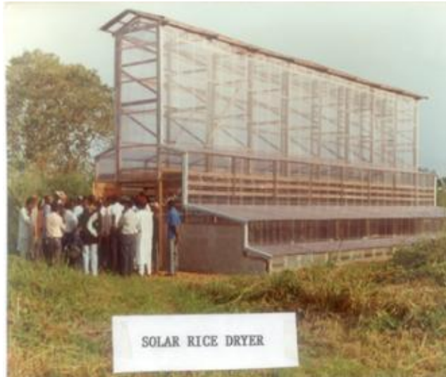
Figure 11: A 2 tonne solar Rice Dryer (NCERD)
