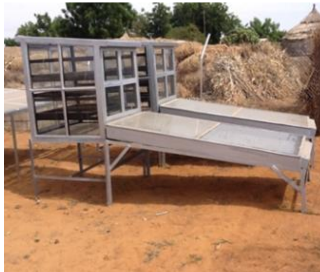
Figure 10: 100kg Solar Dryers installed in Danjawa
