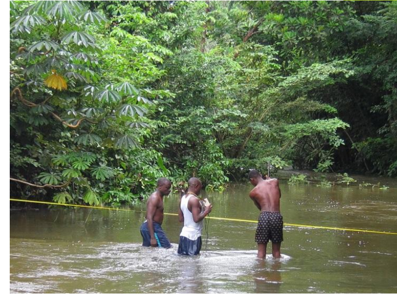
Mechanical Flow Measurement by Current meter for small and medium rivers
