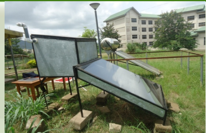
Mixed-mode solar dryer
